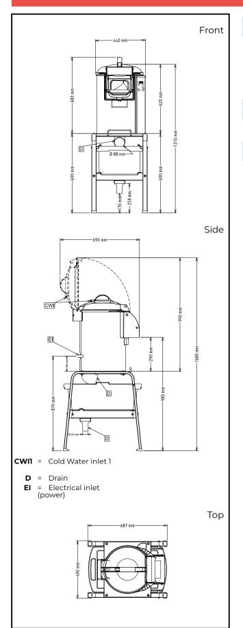
Supply voltage: 603509 (DT10E1) 220-240 V/1N ph/50/60 Hz 200-240/380-440 V/3 603510 (DT10E324) ph/50/60 Hz Electrical power max.: 0.37 kW 0.37 kW **Total Watts:** Capacity: Performance (up to): 160 kg/hour
